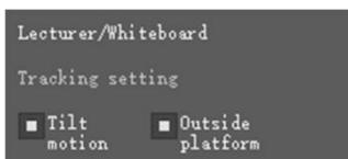
**Tilt motion:** During the tracking process, the camera automatically adjusts the camera's pitch angle according to the target height;
