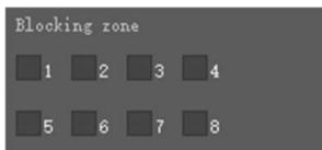
Blocking zone: A maximum of 8 shielding areas can be set, displayed in red boxes, and any shielding area can be canceled separately. The motion objects in the area of the panoramic camera will not be tracked, but the close -up camera can still track the designated characters.
