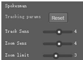
Tracking params: set sensitivity of tracking enable to detect and track. High sensitivity easily, and not lose the object.
