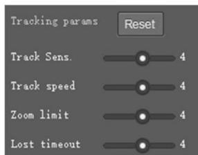
**Tracking sensitivity:** Refers to the tracking motion of the close-up lens that will trigger the scattered amplitude. The higher the sensitivity, the close-range movement will trigger a close-up lens motion.
