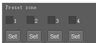
Preset zone: Set the effective area of the preset position, and use the preset area tracking. When the target enters the corresponding preset point area, the camera is transferred to the corresponding preset
