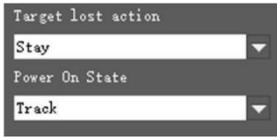
Target Lost Action: used to define the action to be performed if the camera loses the tracked object for a period of time.
